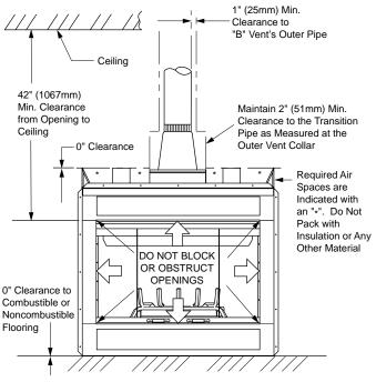
Figure 4 - Minimum Clearances (Front View)
